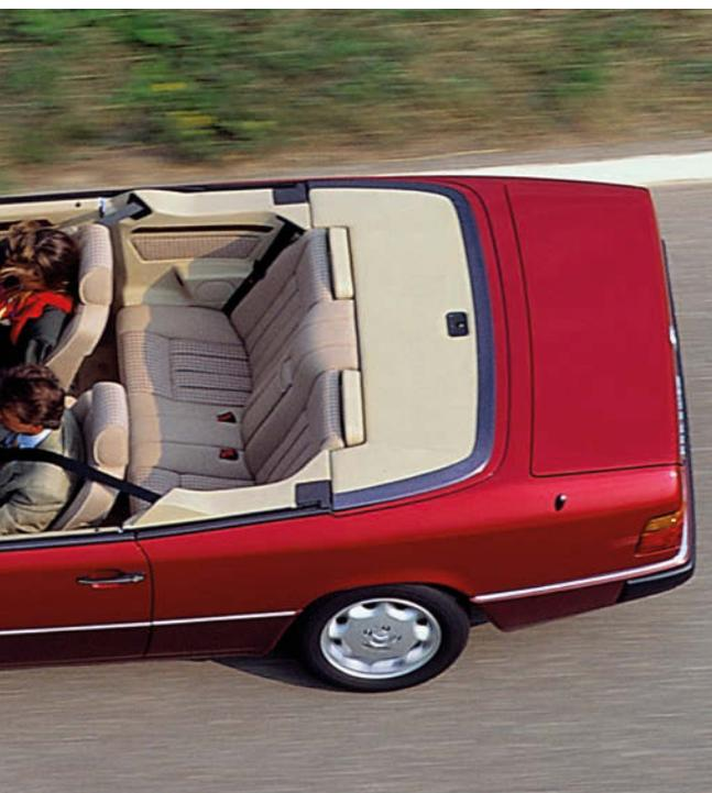
Check too for shrinkage around the edges, make sure the hood pulls taut when raised, but not so taut that securing it becomes difficult. Check the frame too – it shouldn't be too stiff, nor should it rattle once the hood is in position. Correct lubrication is even more important if the hood is electrically operated, as any stiffness can put extra pressure on the electrical circuits and potentially lead to motor damage. If it is electric, check that it raises and lowers correctly too.
