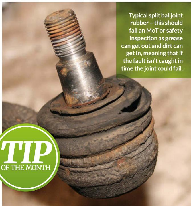
Typical split balljoint rubber – this should fail an MoT or safety inspection as grease can get out and dirt can get in, meaning that if the fault isn't caught in time the joint could fail.
