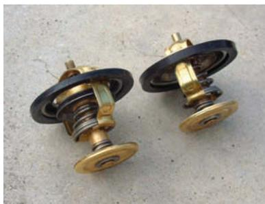
the open position, or the thermostat having been removed. Sometimes a faulty fan will also cause excess cooling – an electric fan that runs all the time, or a viscous coupling mounted on one on which the coupling has failed, meaning the fan turns all the time rather than being able to slip until the engine reaches temperature.
